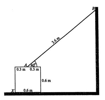
A ladder AB, of length 3.6 m and mass 15 kg, rests in equilibrium at 40° to the horizontal. Its upper end B is in contact with a smooth vertical wall, and its lower end A is in contact with the rough horizontal top surface of a cubical block. The ladder is modelled as a uniform rod lying in a vertical plane perpendicular to the wall (see diagram).
